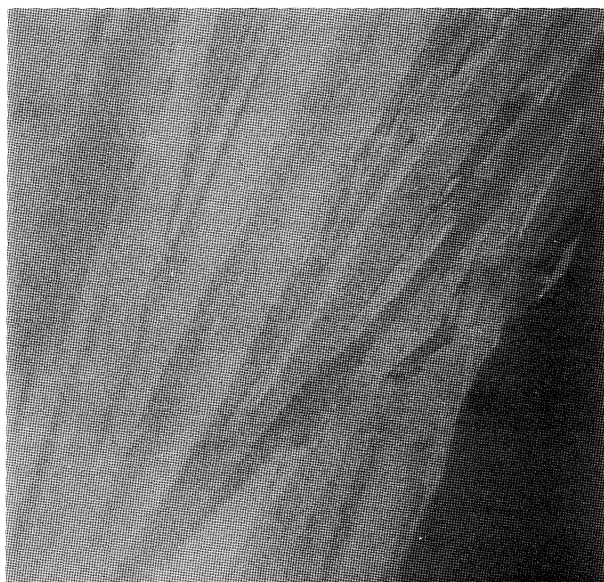
Fig. 5. Photomicrograph of the nematic liquid crystal monomer of 1 at 98 °C between crossed polarizers (magnification: 1×50).
